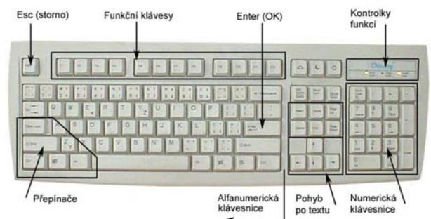
The keyboard is connected to the computer via a serial port PS / 2 or using a universal serial bus (USB), wireless variants are also available.
